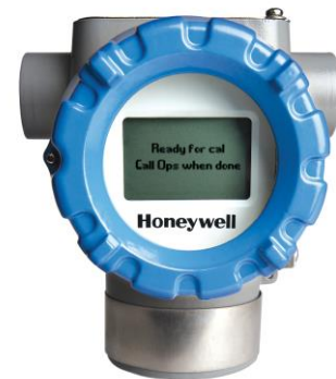
SmartLine STT850 Temperature Transmitter with Advanced Display showing PV and PV Trend for a RTD sensor. The full set of display screens are easily advanced using the local three buttons on the top of the transmitter. Configuration of the transmitter using the three buttons is also fully supported; thereby, avoiding the need of a handheld device.
