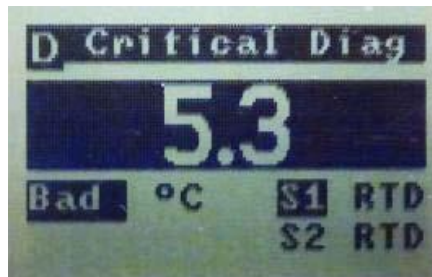
SmartLine STT850 Temperature Transmitter with Advanced Display showing Bad PV for RTD sensor 1. STT850 is available with a dual input option and RTD sensor 2 could serve as a redundant input.
