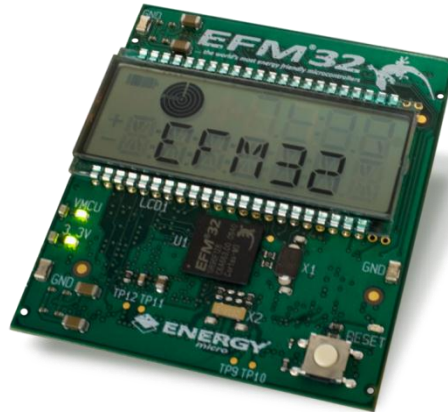
Figure 7: EFM32 directly driving a 160 segment LCD display
