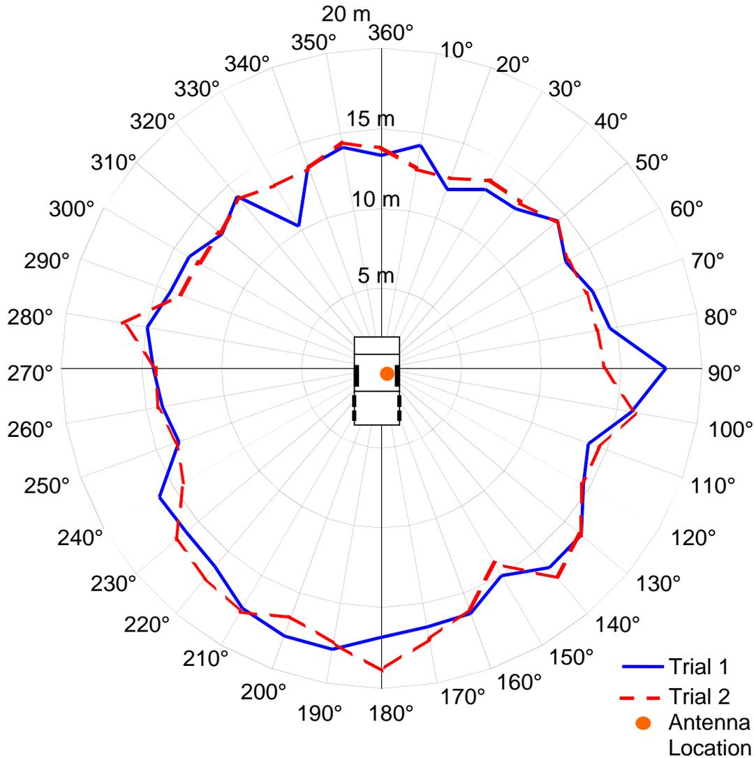
**Figure 6:** Active proximity warning zone for a specific alert range
