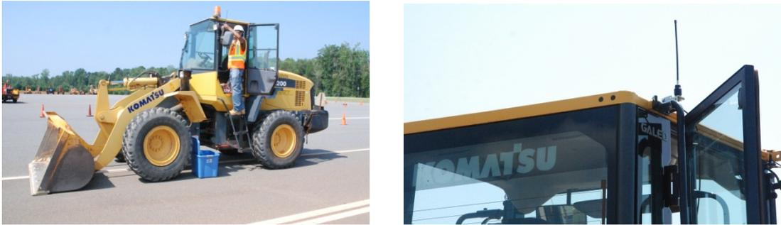
**Figure 4:** Mounting position of an EPU antenna on a wheel loader cabin (left); detail view of antenna location (right)
