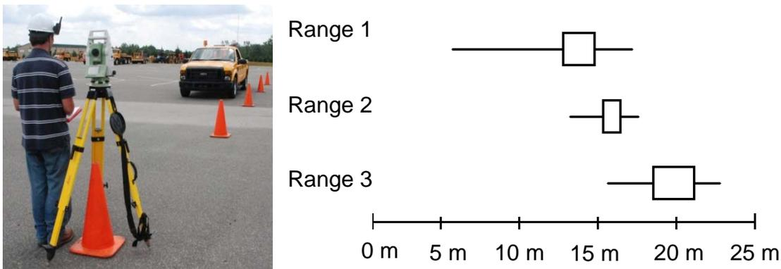
**Figure 7:** Static worker and dynamic equipment experiment (left) and box plot of proximity detection distance for each personal tag (right)
