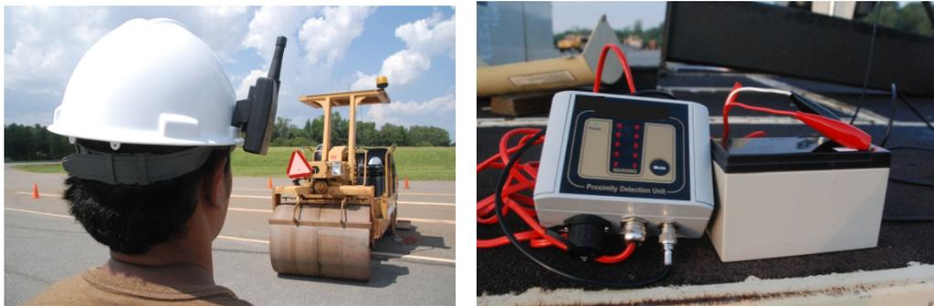
**Figure 1:** PPU device installed on a ground worker's hard hat (left), EPU device installed on an asphalt paver (right) with alert activated
