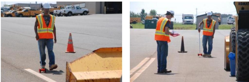
**Figure 5:** Measurement of the alert distance (left); Test person recording the measured alert distance (right)
